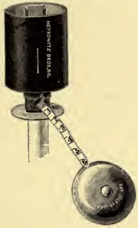
FIG. 112.—A simple arrangement for determining the near point (Landolt).
